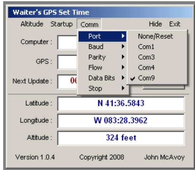
**COMM** - Select the serial port parameters These are the standard Port Number, Baud rate, flow, etc, etc. Most GPS receivers will transmit at 4800 baud, No Parity, No Flow control, 8 Data bits, and 1 stop bit.
